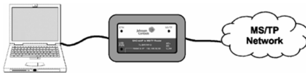
Figure 6: Setup for Initial IP Address Configuration
